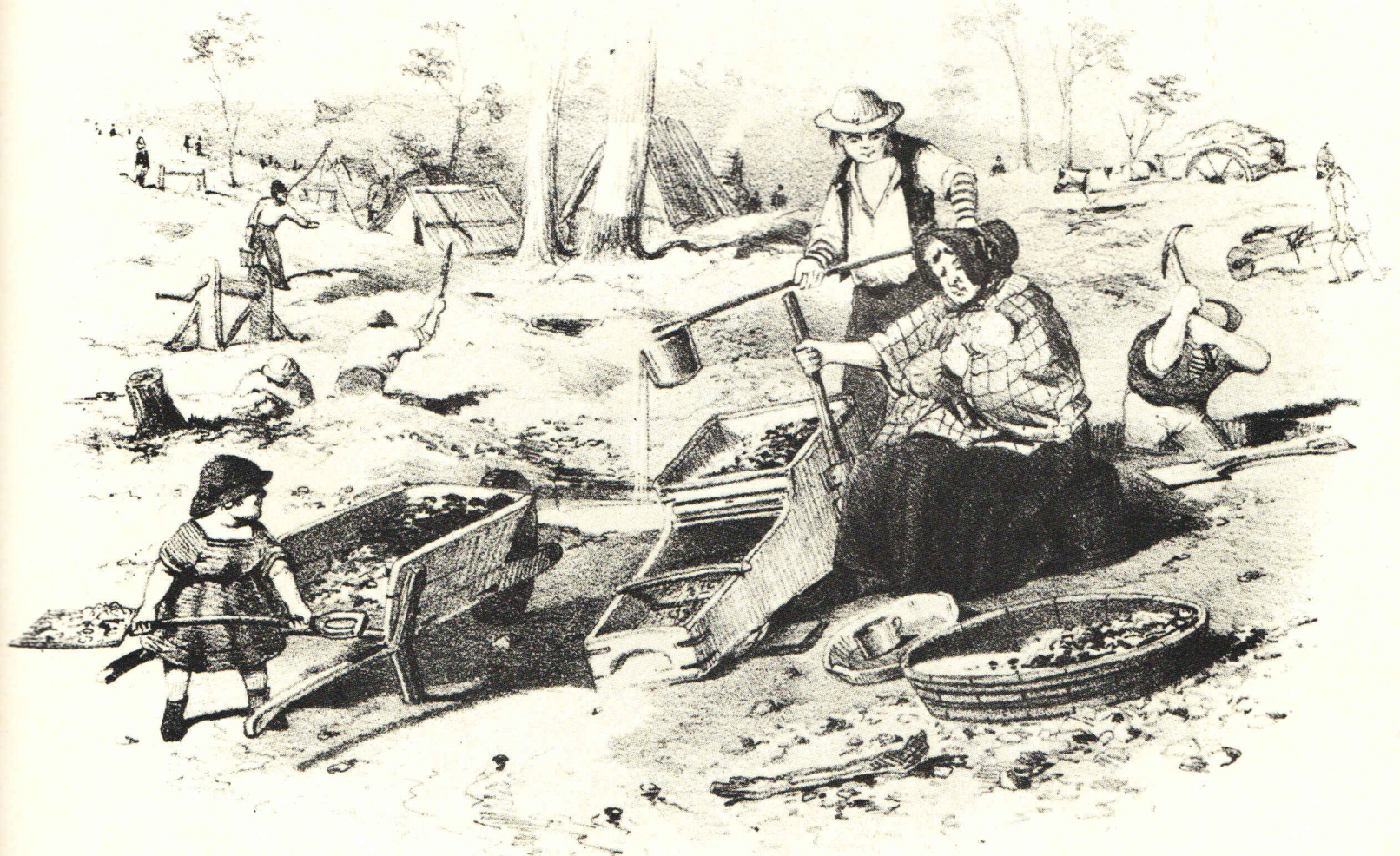
Mining was often a family affair. Here a digger excavates soil, his son washes it, his wife rocks the cradle to shake out the gold and his small daughter struggles with a spade.
